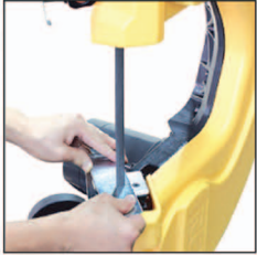
Contour cutting for small steel material
