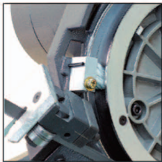
Brush removes waste powder to reduce slippage of saw blade.
